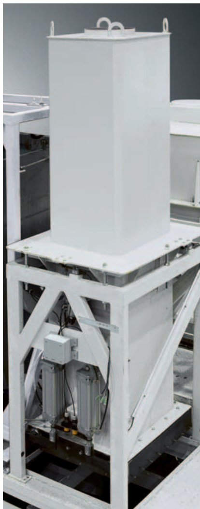
Ice weighing system for weighing of flake ice.
