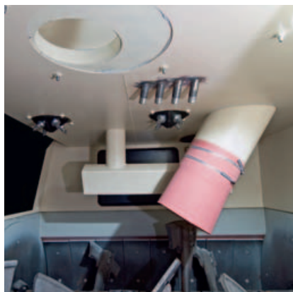
Nozzle heads for cleaning of the mixer.
