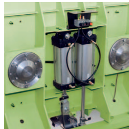
The pneumatic discharge gate operation.
