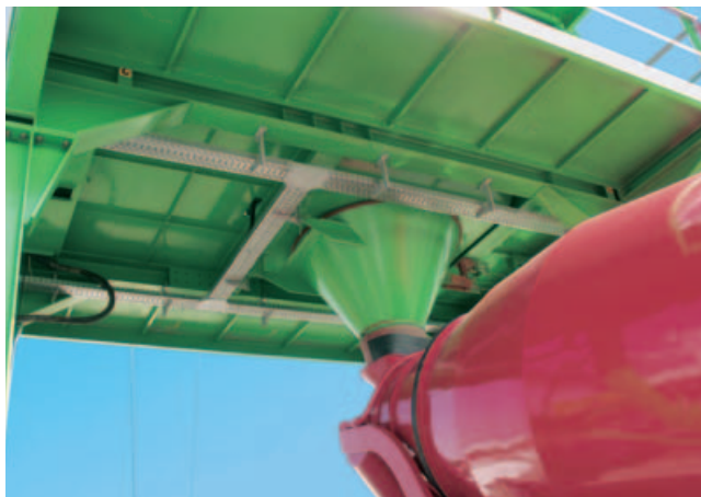
The mixer discharge for filling truck mixers.
